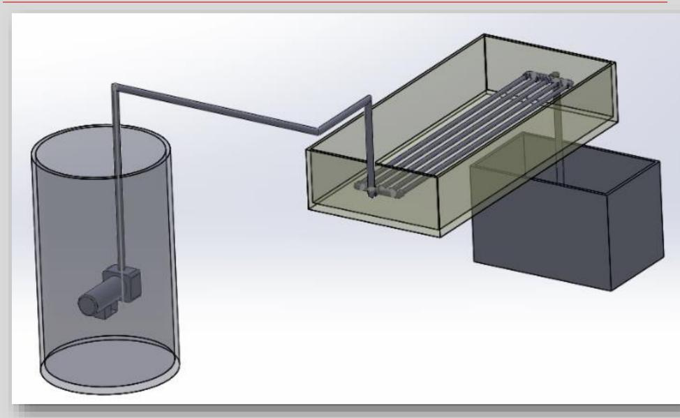
The testing apparatus will provide the team a means to validate the predictive engineering in the software. It will consist of a heated water reservoir, water pump, keel cooler, and water bath. It will simulate the worst case operating scenario for a vessel, wide open throttle for a vessel which is stationary.
